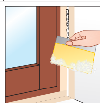
Finish the sealing with a wet spatula
